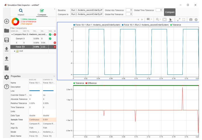
7 Determine whether the numerical discrepancies are significant by specifying an absolute relative tolerance value. For this tutorial, set the global absolute tolerance to 1e-12. In the upper-right corner click the More button. In the dialog box, under Global Tolerances, set Absolute to 1e-12. Then, click Compare. The comparisons for X and Force: f(t):1 are within tolerance.
