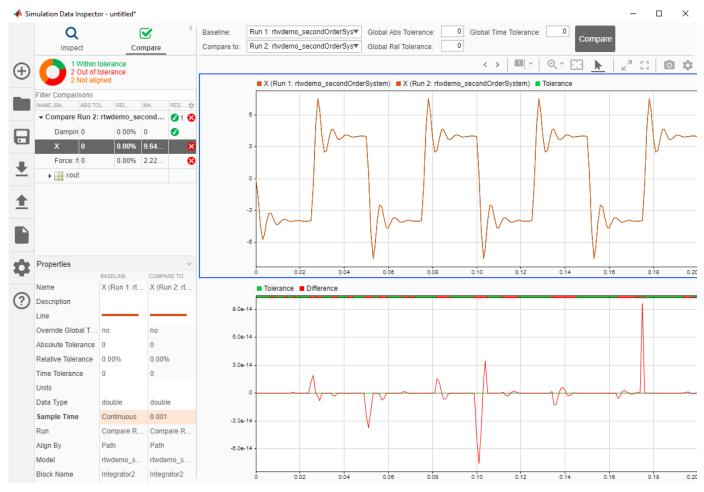
6 Inspect the comparison plot for Force: f(t):1. Under File Comparisons, select the row for Force: f(t):1.
