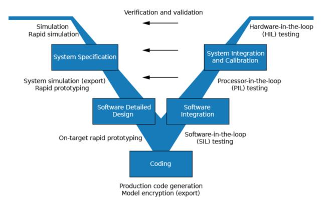
Depending on your application and its role in the process, you might focus on one or more of the steps called out in the V-model or repeat steps at several stages of the V-model. Code generation technology and related products provide tooling that you can apply to the V-model for system development. For more information about how you can apply MathWorks code generation technology and related products to the V-model process, see "Types of Simulation and Prototyping in the V-Model" on page 1-6.
