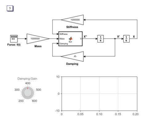
The model implements a second-order physical system called an ideal mass-spring-damper system. Gain blocks represent components of the system equation: Mass, Stiffness, and Damping. The equation for the system is mX'' + cX' + kX = f(t).
